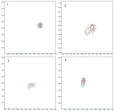
FIGURE 9: Overlay of 2D  $^{1}H-^{15}N$  HSQC spectra (expansions for four crosspeaks) for the titration of DHPR with NADH. Full spectrum is in Supporting Information. DHPR was present at 800  $\mu$ M and NADH was present at 0 (black), 20 (red), 40 (green), 100 (blue), 200 (yellow), 400 (magenta) and 2000 (cyan)  $\mu$ M. Peak #1 is from Trp253.
