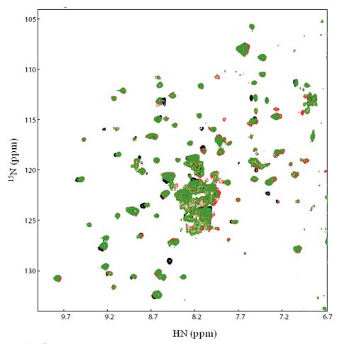
FIGURE 11: Overlay of 2D  $^{1}H^{-15}N$  HSQC spectra of 0.8 mM DHPR (black), 0.8 mM DHPR + 2.0 mM CRAA (red) and 0.8 mM DHPR + 2.0 mM CRAA + 2.0 mM PDC (green).
