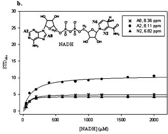
FIGURE 3: STD titration of DHPR ( $\pm$ PDC) with NADH. STD intensities were recorded for three NADH protons, and fitted to the equation: STD<sub>obs</sub> = -STD<sub>max</sub>/(1 + ([NADH]/ $K_d$ )<sup>n</sup>) + STD<sub>max</sub>. (a) STD titration of DHPR with NADH without PDC bound. (b) STD titration of the DHPR •PDC complex with NADH. The inset is the NADH structure with A8, A2 and N2 protons assigned.
